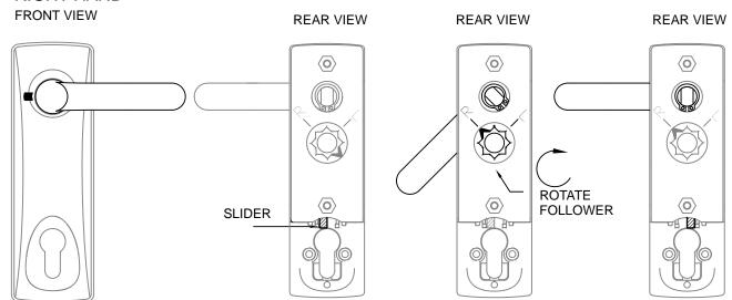
USING A 2.5MM ALLEN KEY LOOSEN THE GRUB SCREW AND REMOVE THE HANDLE. REPLACE AS SHOWN AND RETIGHTEN THE GRUB SCREW LOOKING AT THE LOCK FROM THE REAR, MOVE THE SLIDER TO THE LEFT HOLD THE HANDLE IN THE DOWNWARD POSITION AND ROTATE THE FOLLOWER CLOCKWISE UNTIL THE ARROW ALIGNS WITH THE LETTER (R) RELEASE THE HANDLE AND MOVE THE SLIDER TO THE RIGHT
