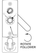
HOLD THE HANDLE IN THE DOWNWARD POSITION AND ROTATE THE FOLLOWER ANTI-CLOCKWISE UNTIL THE ARROW ALIGNS WITH THE LETTER (L)
