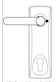
USING A 2.5MM ALLEN KEY LOOSEN THE GRUB SCREW AND REMOVE THE HANDLE, REPLACE AS SHOWN AND RETIGHTEN THE GRUB SCREW
