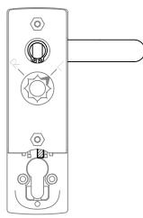
RELEASE THE HANDLE AND MOVE THE SLIDER TO THE RIGHT
